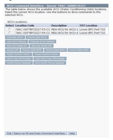
16. Identify all WCU's installed in the system using image and location code information listed below.
