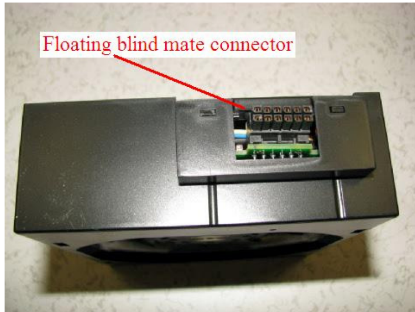
Figure 38 Fan blind mate connector
