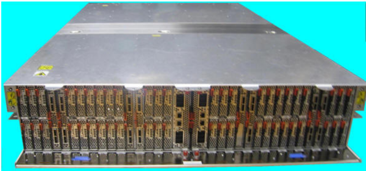
Figure 9 Disk Enclosure Photo (Front View – showing 48 Drive Carriers, 8 Port Cards, and 2 DCCAs)
