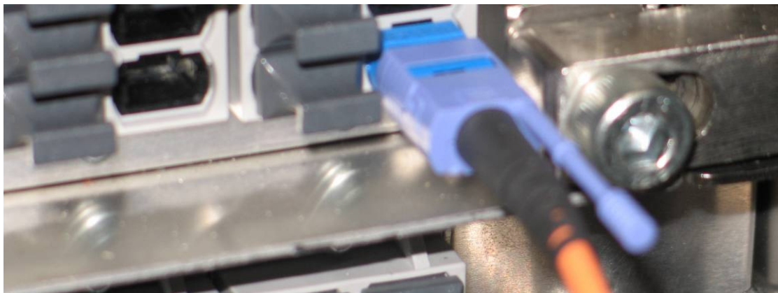
Figure 15 Individual D-Link Connector with push/pull tab on upper right
