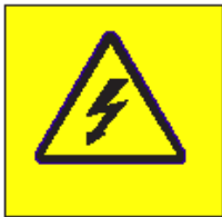
Figure 1 Hazardous Voltage, Current, or Energy
