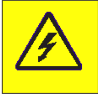
Figure 5 Hazardous Voltage, Current, or Energy
