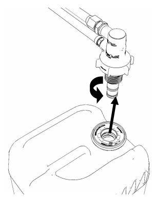
29. Replace the inner cap into the white system water container insert. Turn inner cap clockwise with a large screwdriver. Power775 Bulk Power Distributor (BPD) Fill and Drain Tool Procedures: ---- FDT Tank Drain Procedure ----
