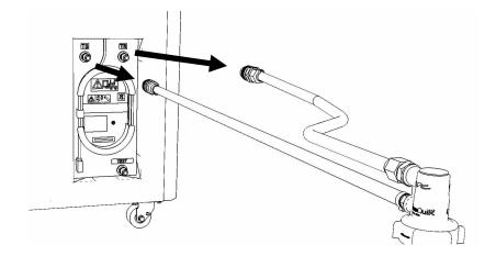
28. Remove large white threaded insert of **THA** from the system water container. Turn **slowly** counterclockwise until removed.
