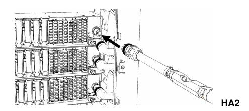
23. Ensure all hose connections are made properly and securely. Verify hoses are connected as outlined in the schematic below. Power775 CEC Fill and Drain Tool (FDT) Procedures ---- CEC Pressure Test Procedure ----
