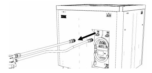
28. Remove large white threaded insert of **THA** from the system water container. Turn **slowly** counterclockwise until removed.
