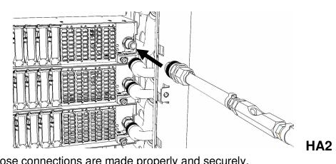
25. Ensure all hose connections are made properly and securely.
