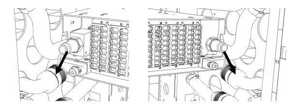
20. Remove hose assembly **HA1** from the upper tool storage compartment.
