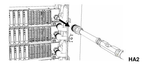
34. Connect the system manifold hoses to the CEC water connections.
