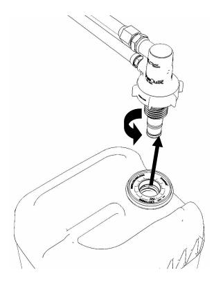
29. Replace the inner cap into the white system water container insert.
