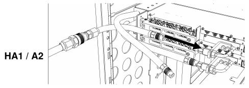
24. Connect the unattached end *with sight glass* of hose assembly **HA2** to the other adapter **A2**.
