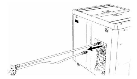
27. Disconnect the **Upper THA Hose** from the **TS** connection on the front panel of the FDT.
