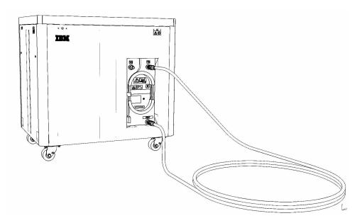
20. Ensure all water connections are made properly and securely.
