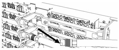
19. Remove hose assembly **HA1** from the upper tool storage compartment.
