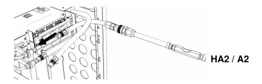
25. Ensure all hose connections are made properly and securely. Verify hoses are connected as outlined in the schematic below.
