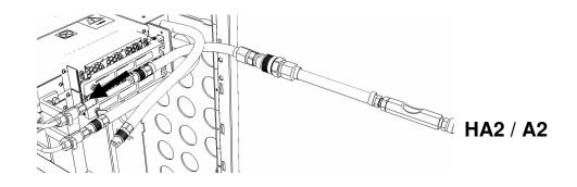
25. Ensure all hose connections are made properly and securely.
