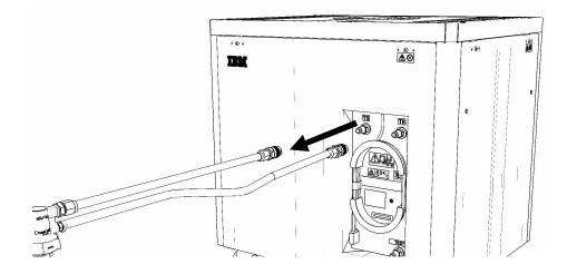
28. Remove large white threaded insert of **THA** from the system water container. Turn **slowly** counterclockwise until removed.
