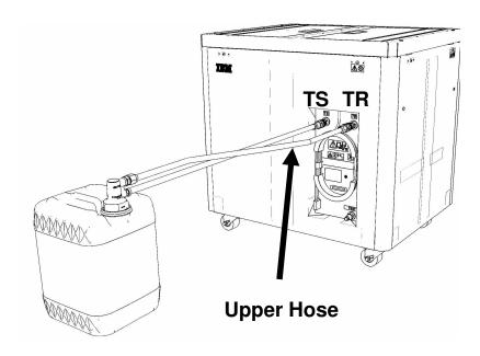
22. Ensure all water connections are made properly and securely.
