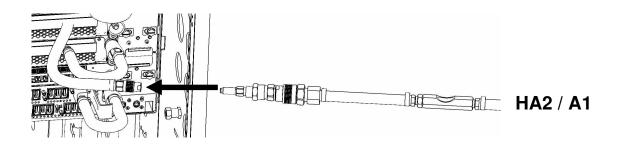
25. Ensure all hose connections are made properly and securely.
