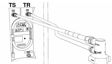
22. Ensure all water connections are made properly and securely.
