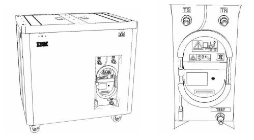
5. Unwrap the FDT UPIC cable from the storage loop on the FDT.
