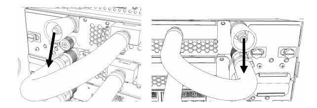
19. Remove hose assembly HA1 from the upper tool storage compartment.
