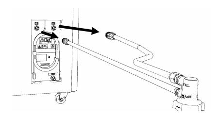
28. Remove large white threaded insert of **THA** from the system water container.
