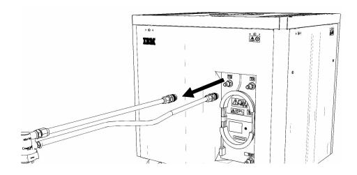
28. Remove large white threaded insert of **THA** from the system water container.
