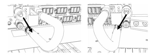
19. Remove hose assembly HA1 from the upper tool storage compartment.
