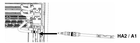
25. Ensure all hose connections are made properly and securely.
