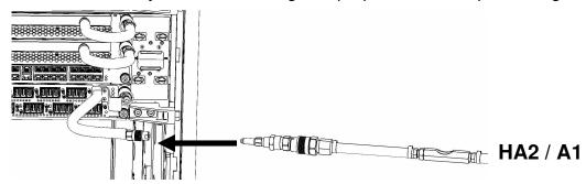
23. Ensure all hose connections are made properly and securely.
