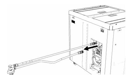
27. Disconnect the **Upper THA Hose** from the **TS** connection on the front panel of the FDT.
