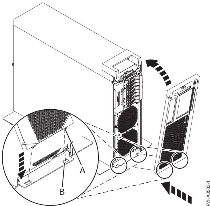
Figura 18. Instalando a Tampa Frontal
