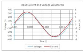
Input AC Current Waveform (ITHD = 4.24%, 50% Load)
