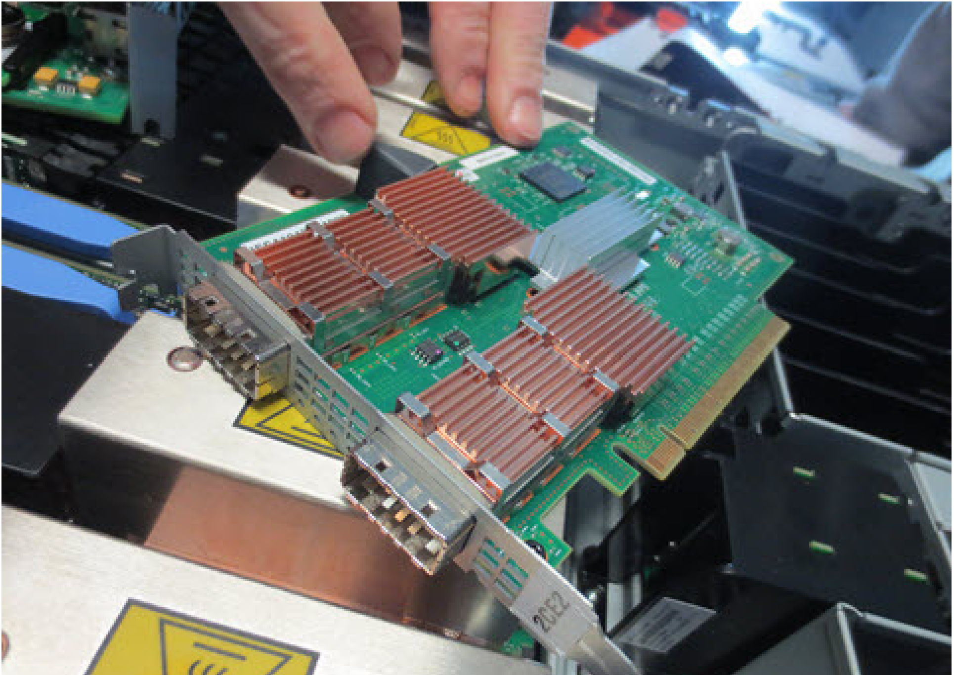
POWER8 I/O Drawer adapter for a pair optical cables to the same drawer half
