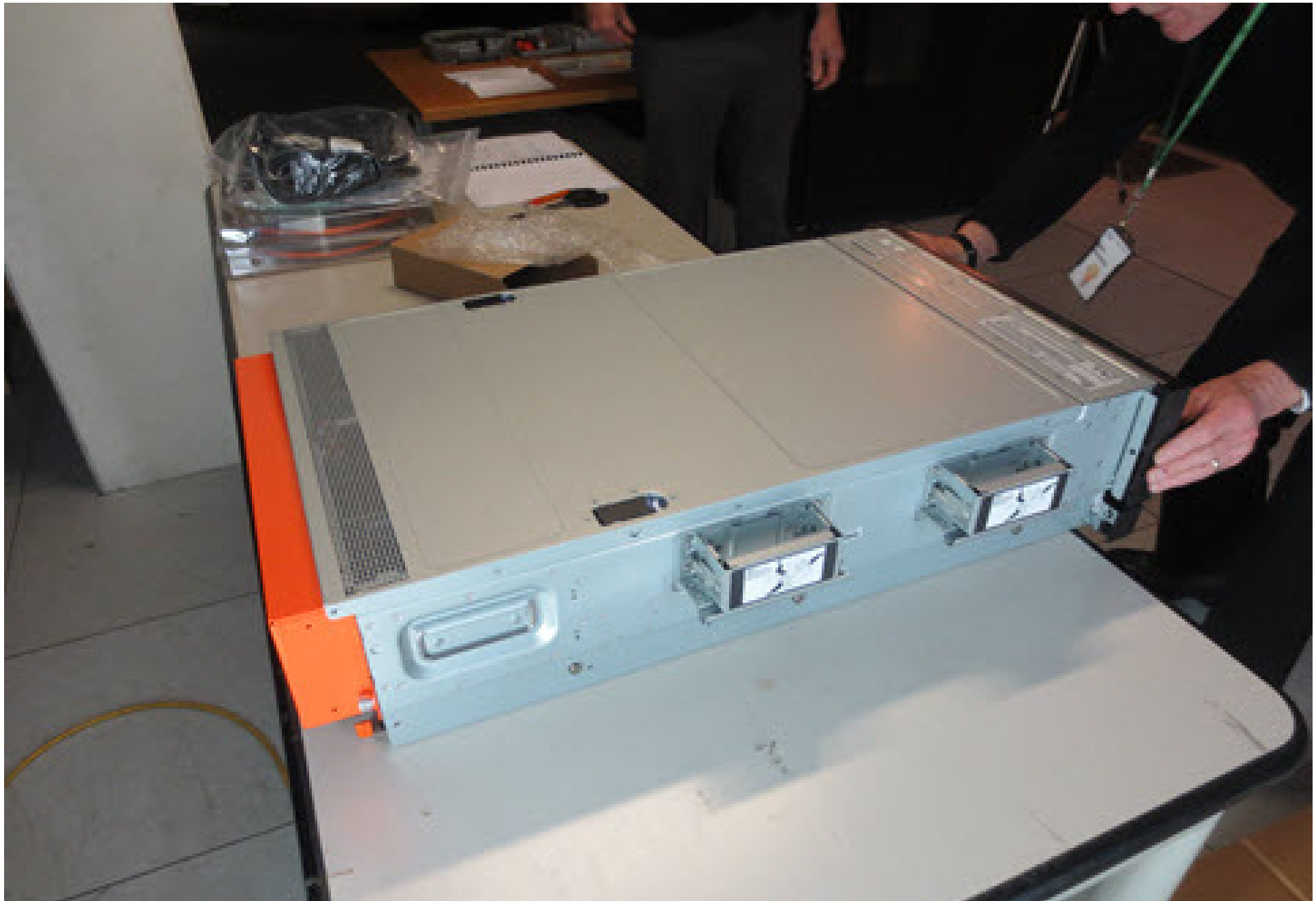
We placed it temporarily on a table. Note orange I/O protection
