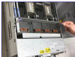
Remove the fan tray to access SAS Raid adapters
