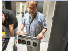
Remove the fan tray to access SAS Raid adapters
