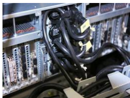
Four power cords Plugs do NOT go through brackets
