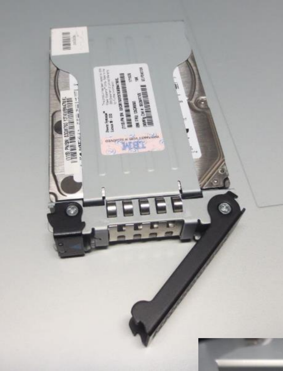
IBM Winchester SAS Disk 1.8 TB in a strong metal case
