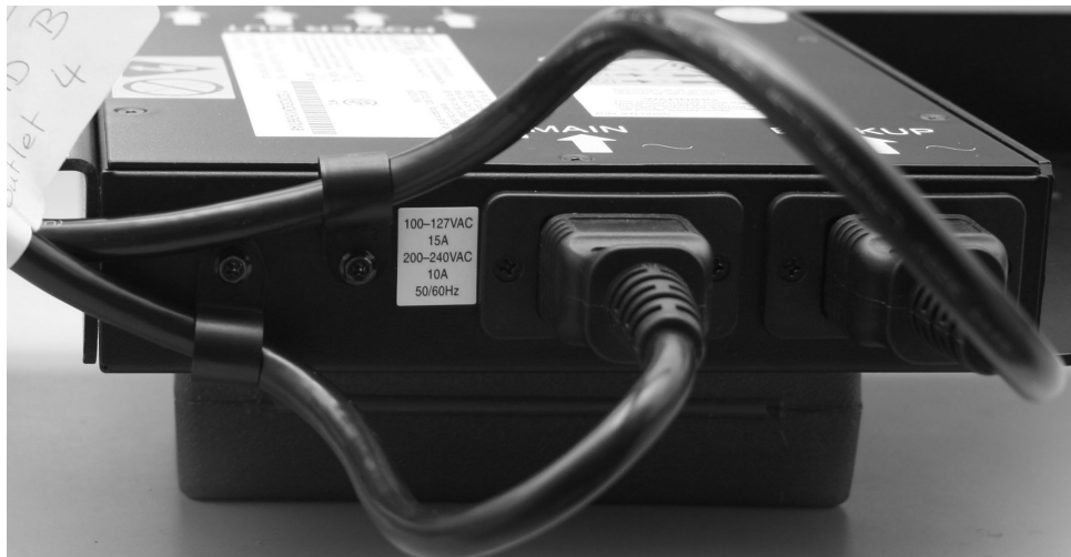
Figure 5. Power cable clips
