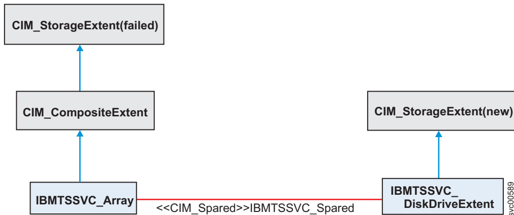
Figure 13. Association during failure
