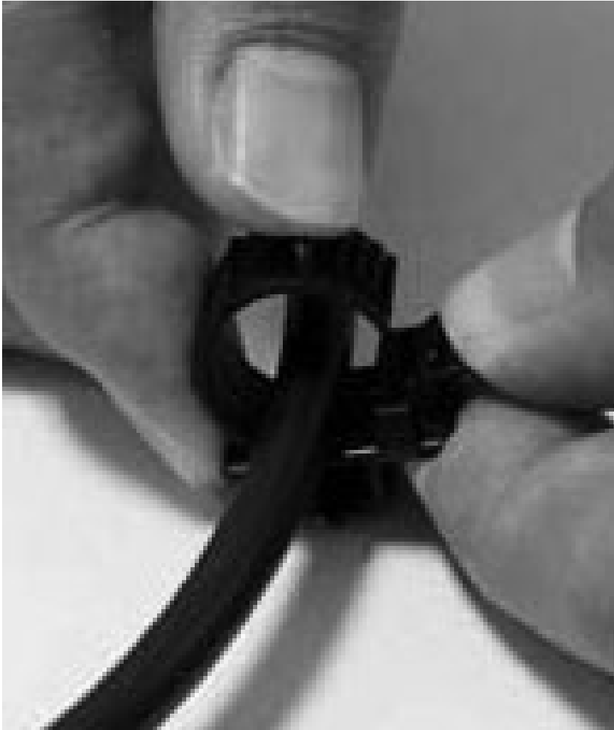
Figure 15. Unlocking the cable retention bracket
