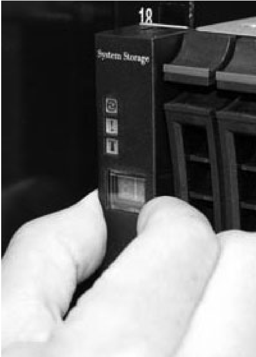
Figure 10. Removing the enclosure end cap
