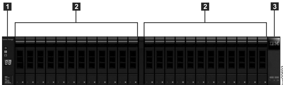
Figure 1. 24 drives and two end caps
