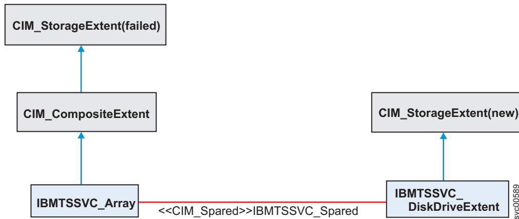
Figure 13. Association during failure
