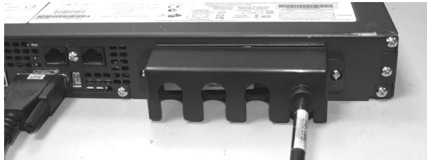
Figure 296. 2145 UPS-1U power cable-retention bracket
