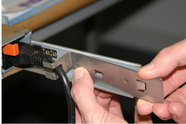
Figure 36. Attaching the cable retention bracket to the SAN Volume Controller 2145-8F4 power cable
