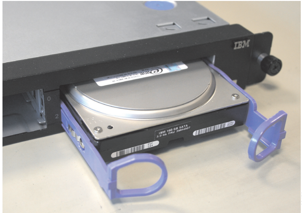
Figure 108. SAN Volume Controller 2145-8A4 SATA disk drive
