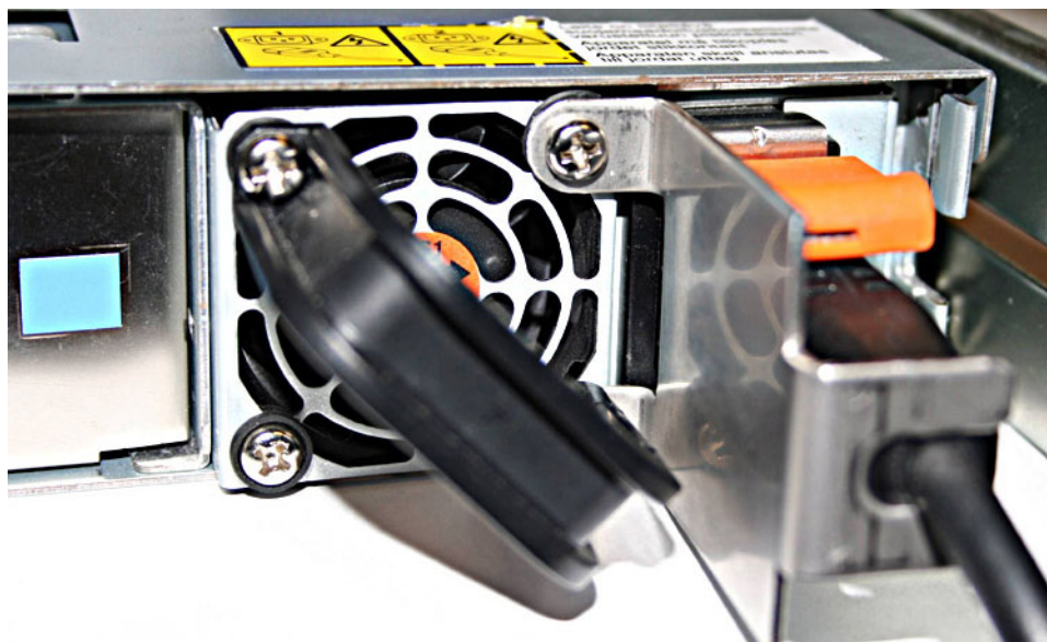
Figure 26. The SAN Volume Controller 2145-8G4 with the cable-retention bracket attached
