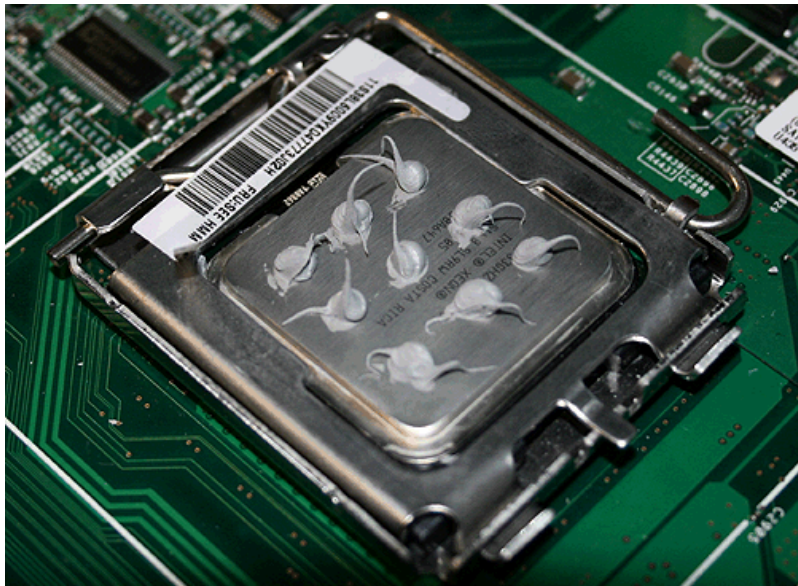
Figure 288. Complete set of nine thermal grease dots on the microprocessor
