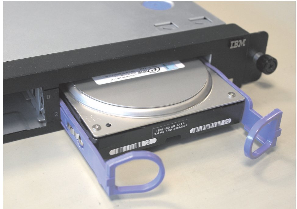
Figure 101. SAN Volume Controller 2145-8A4 SATA disk drive
