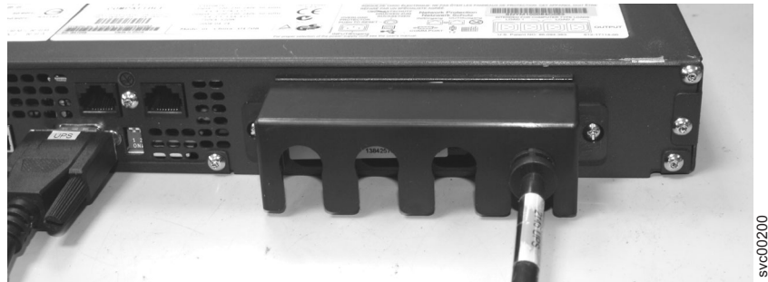
Figure 309. The 2145 UPS-1U cable retention bracket connected to the 2145 UPS-1U
