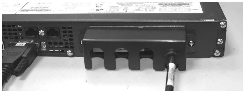
Figure 297. 2145 UPS-1U power cable-retention bracket
