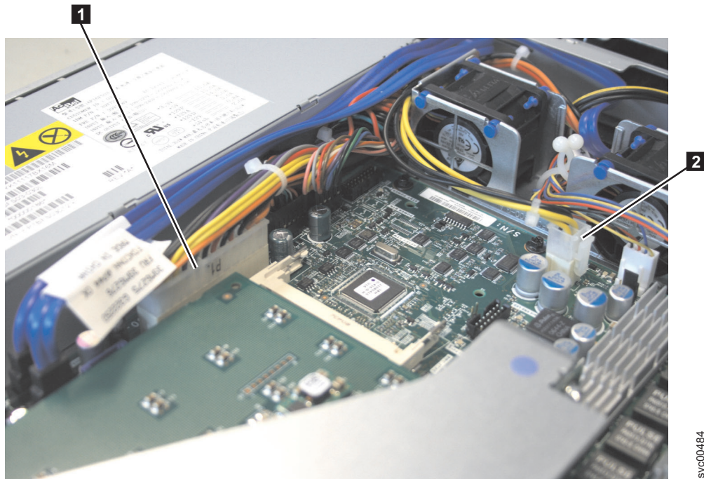
Figure 160. SATA connectors on the SAN Volume Controller 2145-8A4 system board
