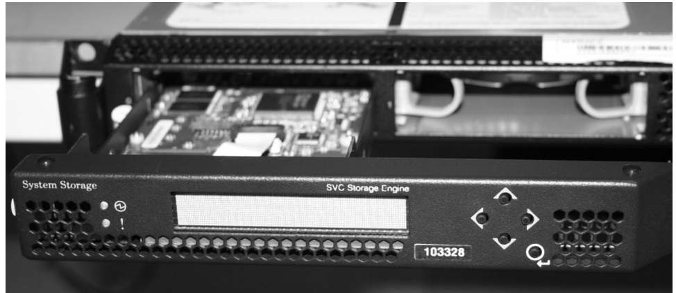
Figure 90. SAN Volume Controller 2145-8G4 service controller
