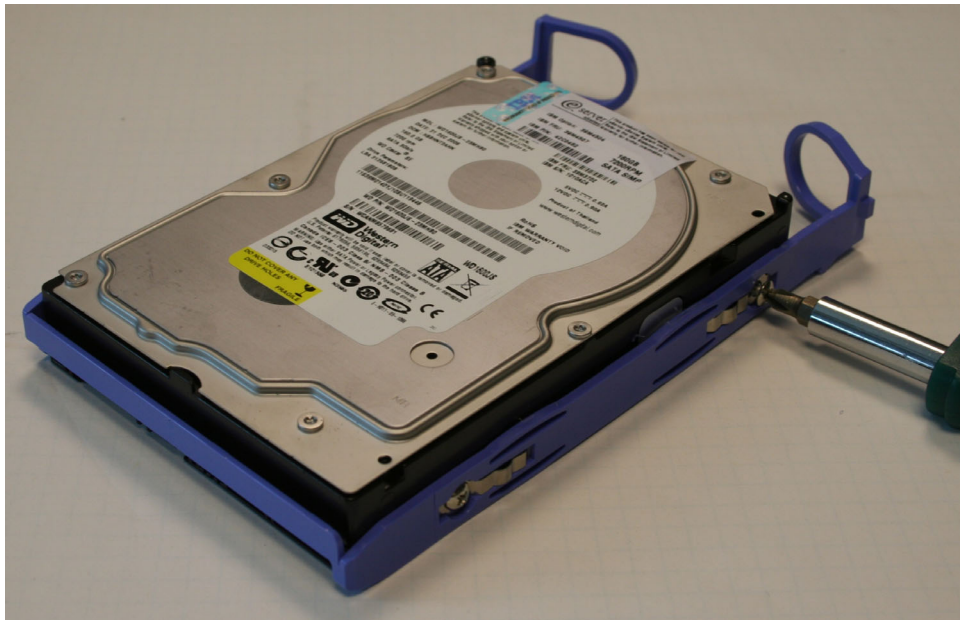
Figure 112. Attaching the rails assembly to the SATA disk drive for the SAN Volume Controller 2145-8A4 and the SAN Volume Controller 2145-8G4
