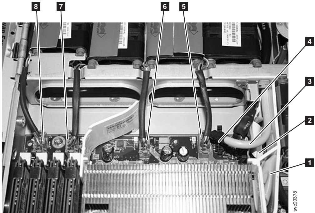
Figure 290. Connectors on the right front side of the SAN Volume Controller 2145-8G4 system board
