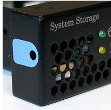
Figure 83. SAN Volume Controller 2145-8G4 service controller release button
