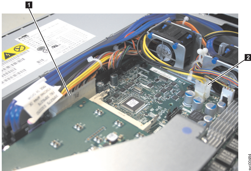
Figure 151. SATA connectors on the SAN Volume Controller 2145-8A4 system board
