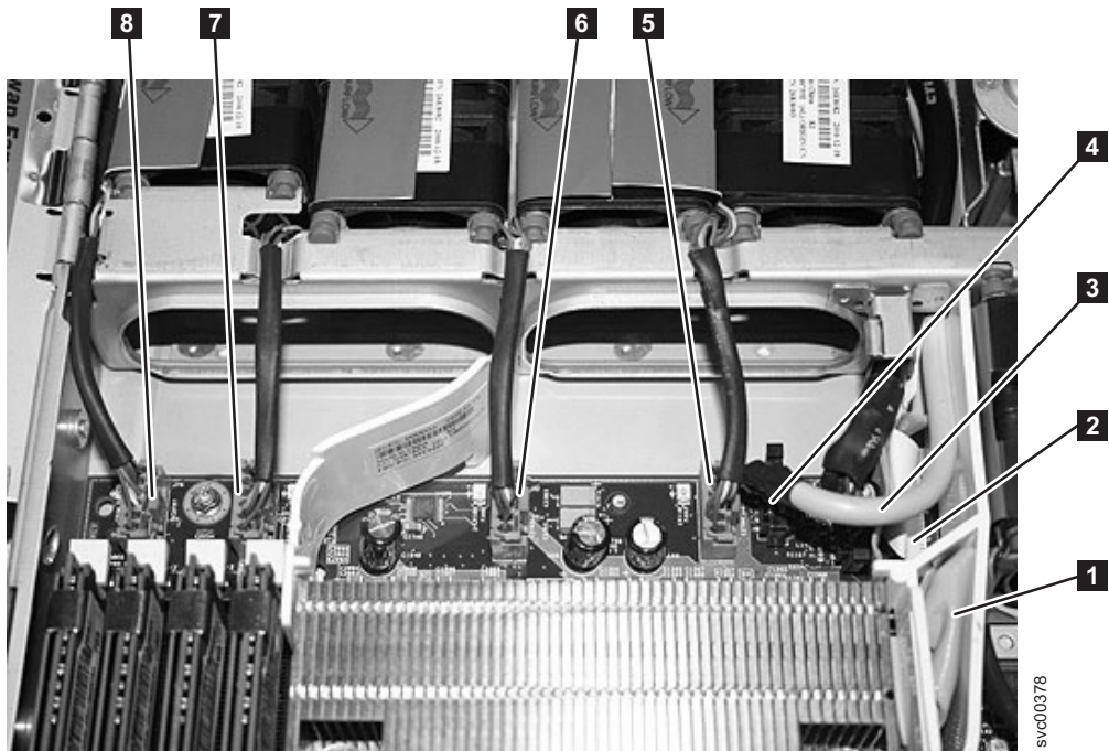
Figure 273. Connectors on the right front side of the SAN Volume Controller 2145-8G4 system board
