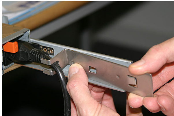
Figure 45. Attaching the cable retention bracket to the SAN Volume Controller 2145-8F4 power cable
