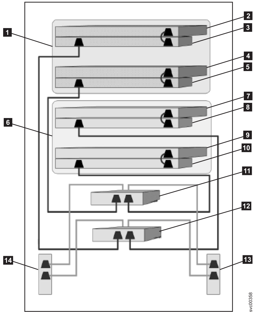
Figure 17. A four-node SAN Volume Controller cluster with the redundant ac-power switch feature
