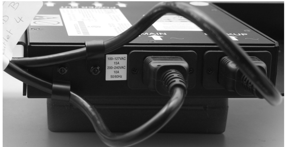
Figure 5. Power cable clips
