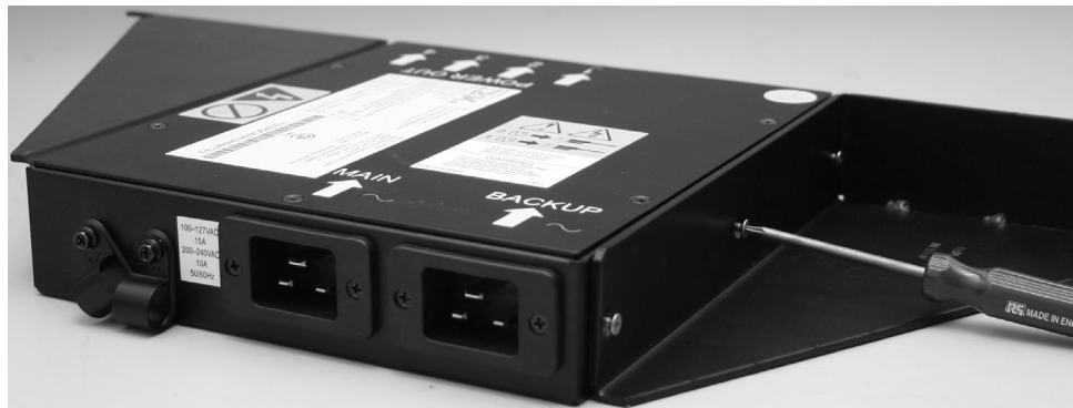
Figure 4. Attaching the mounting plates
