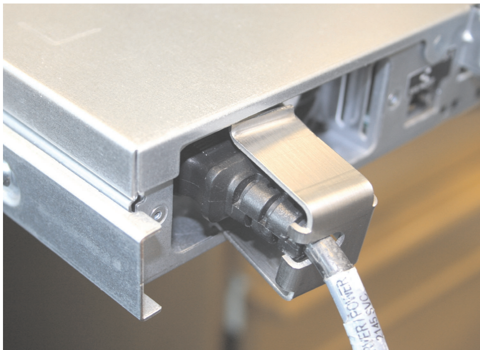
Figure 30. Installing the SAN Volume Controller 2145-8A4 cable retention bracket
