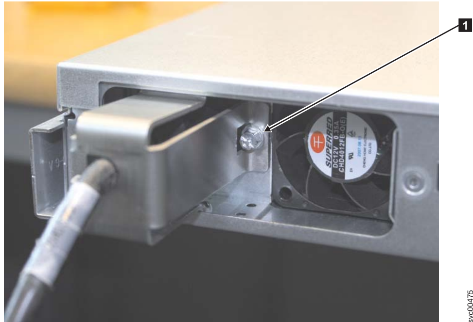
Figure 30. SAN Volume Controller 2145-8A4 with the cable retention bracket installed
