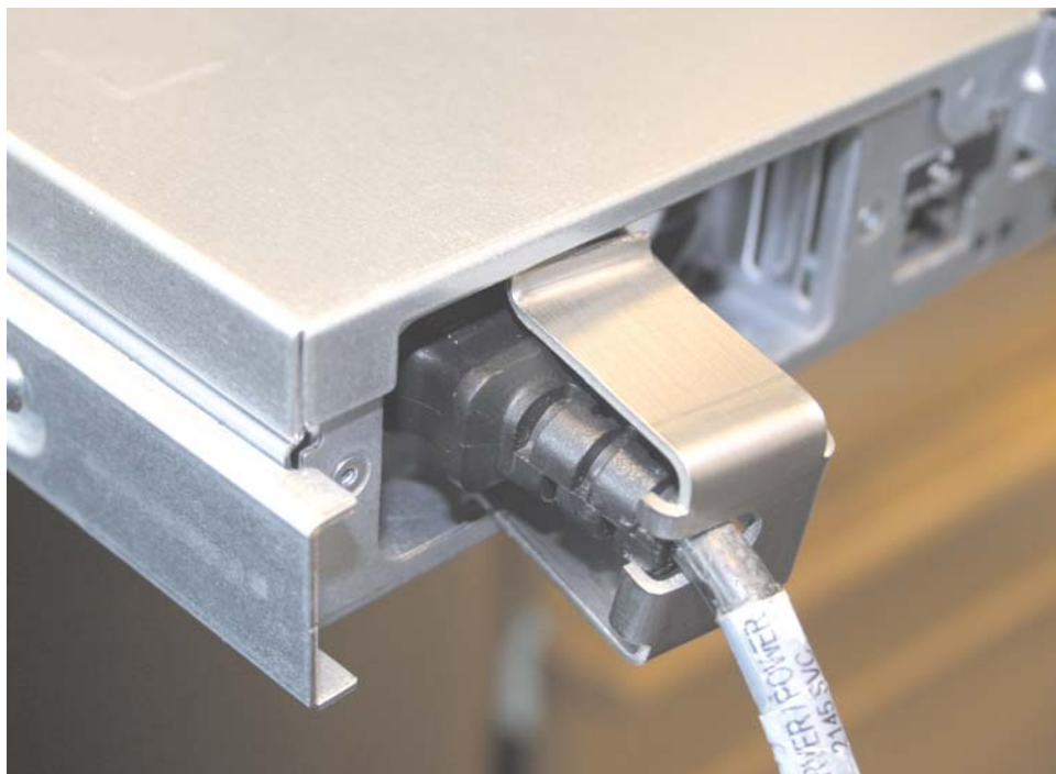
Figure 29. Installing the SAN Volume Controller 2145-8A4 cable retention bracket
