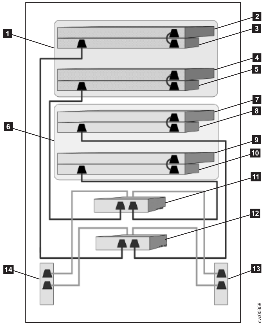
Figure 5. A four-node SAN Volume Controller cluster with the redundant ac-power switch feature
