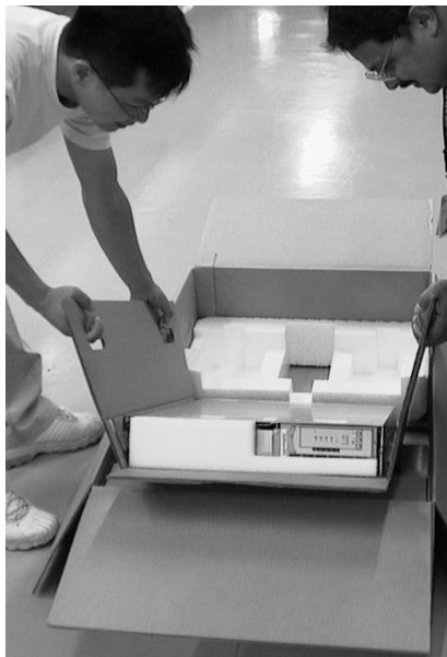
Figure 30. Sliding the 2145 UPS to the end of the carton.
