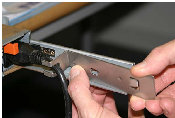
Figure 18. Attaching the cable retention bracket to the SAN Volume Controller 2145-8F4 power cable
