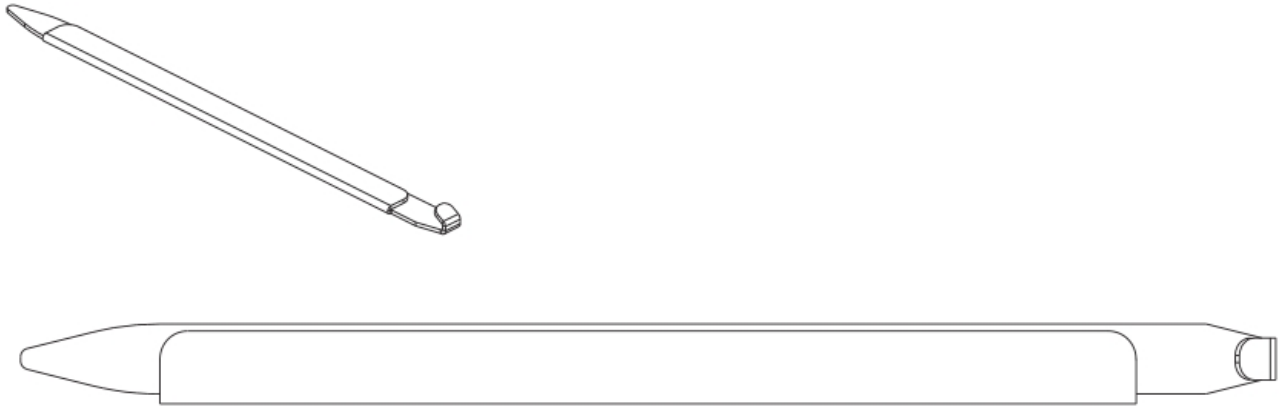
Figure 37. Optical transceiver extraction tool
