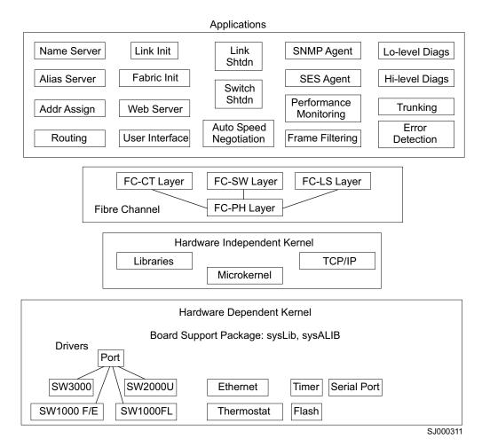
Figure 6. 3534 Model F08 firmware components
