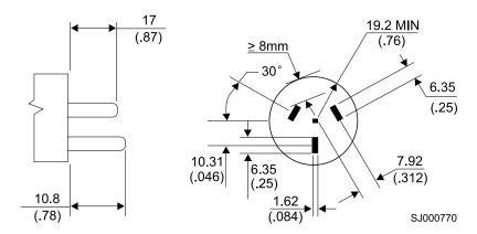
Figure 14. Power cable for Australia
