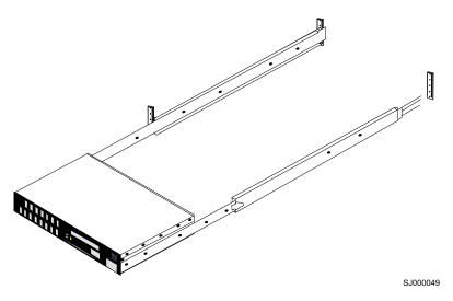
Figure 10. Inserting slides into the rack rails
