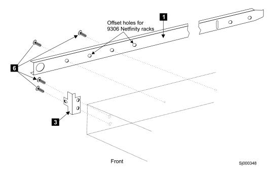
Figure 8. Mounting the moving portion of the slide and the mounting brackets to the switch
