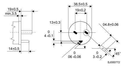
Figure 17. Power cable for Denmark
