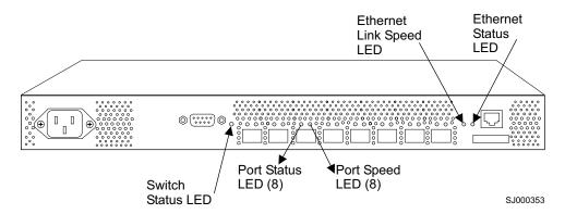
Figure 11. Front panel LEDs
