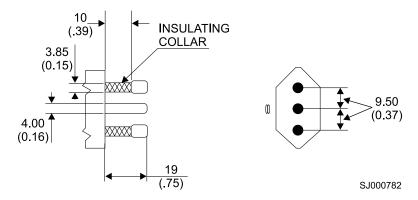
Figure 20. Power cable for Italy
