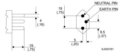
Figure 22. Power cable for Switzerland
