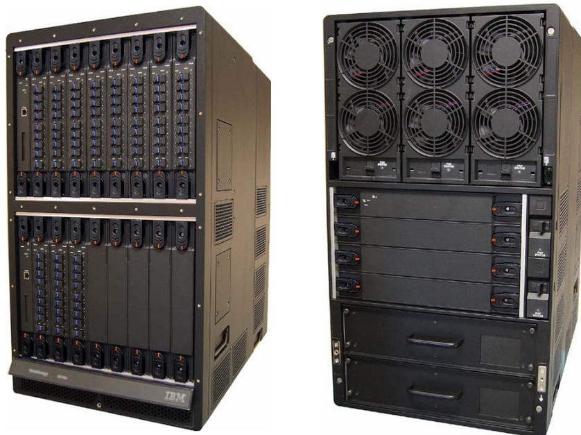
Figure 1. SANC40 cabinet Fibre Channel director, front and rear view
