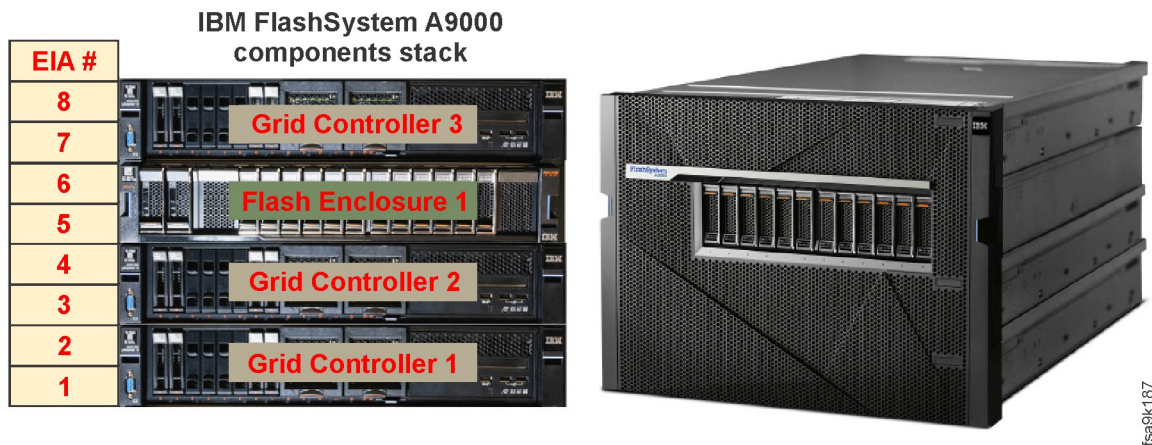
Figure 2. IBM FlashSystem A9000 main components
