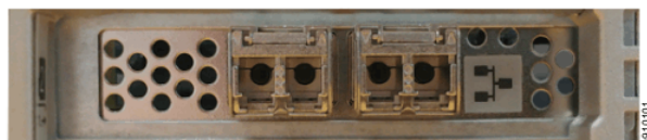
Figure 71. Dual-port 25 Gbps Ethernet host interface adapter ports and LEDs (iWARP)
