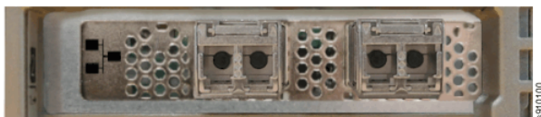
Figure 70. Dual-port 25 Gbps Ethernet host interface adapter ports and LEDs (RoCE)
