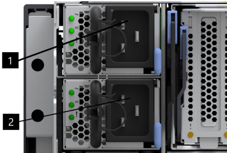
Figure 29. Locate Power Supply Units
