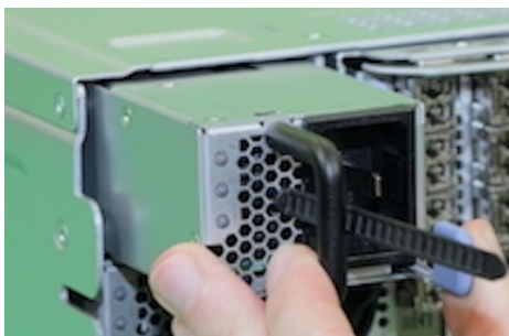
Figure 31. Removing the power supply unit
