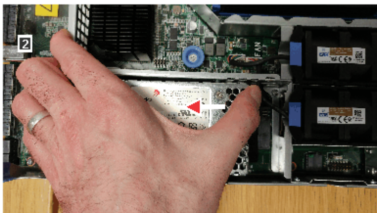
Figure 32. Sliding the node battery out of its position
