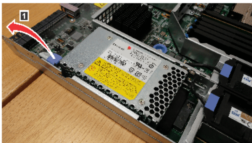
Figure 31. Lifting the latch of the node battery
