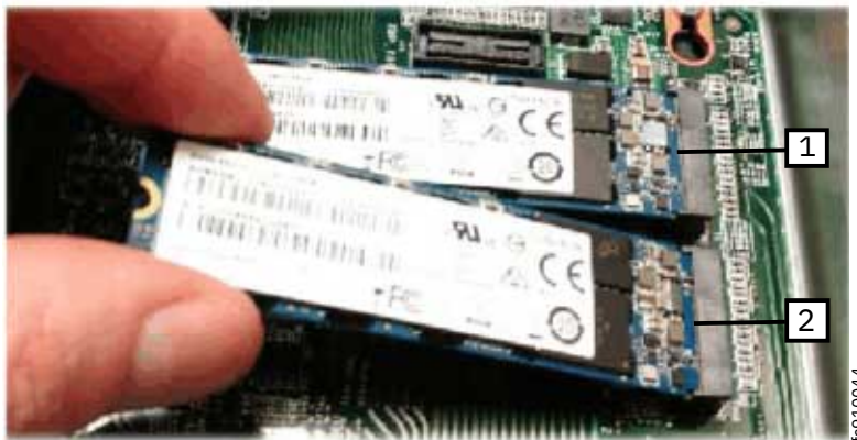
Figure 55. Replacing the boot drive
