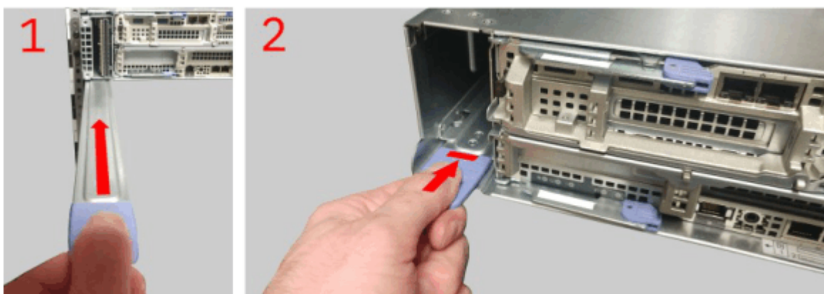
Figure 50. Inserting the new power interposer
