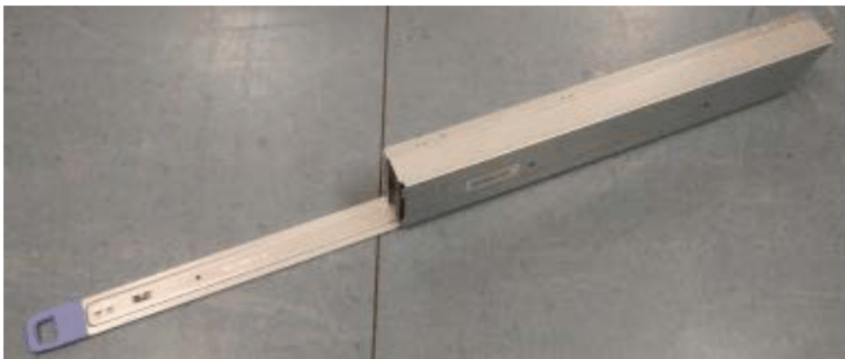
Figure 49. Removing a power interposer
