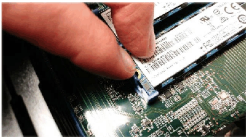
Figure 54. Removing the boot drive
