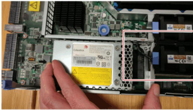
Figure 35. Replacing the node battery
