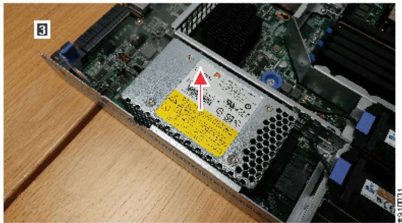
Figure 33. Removing the node battery
