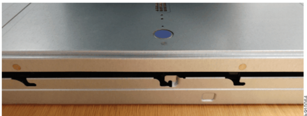
Figure 30. Replacing the node canister cover
