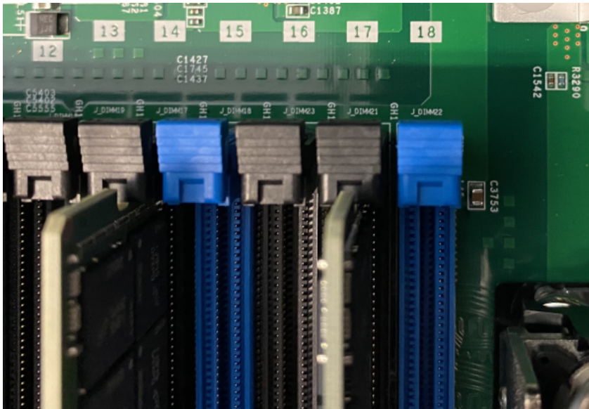
Figure 41. Identifying DIMM locations 13-18
