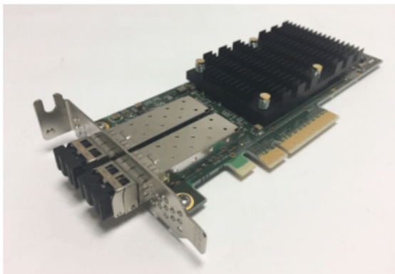
Figure 8. Dual-port 25 Gb Ethernet (iWARP) host interface adapter
