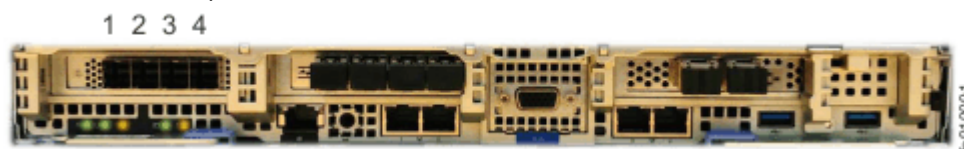
Figure 21. Fibre Channel adapter in adapter slot 1
