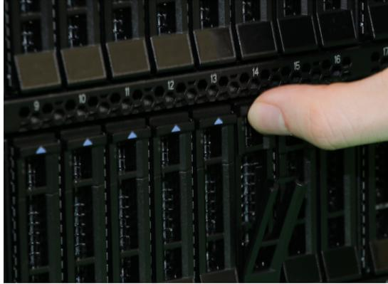
*Figure 72. Unlocking the drive and release latch*
