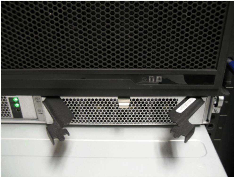
*Figure 159. Install the power supply*
