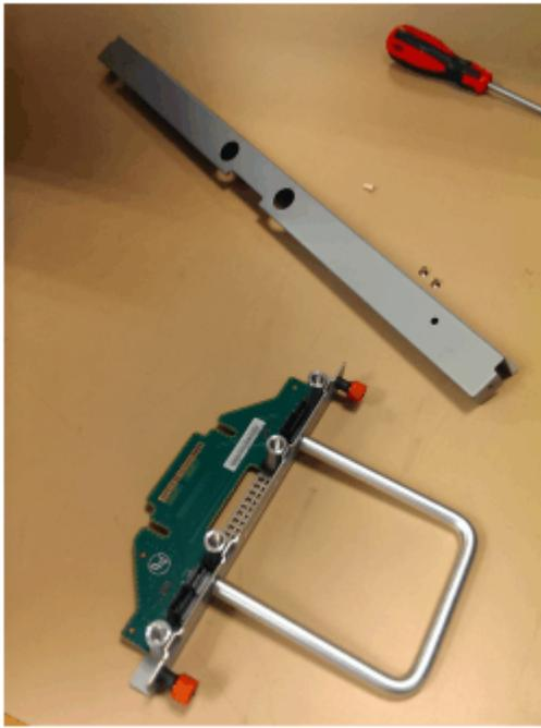
Figure 177. FIB parts removed from the chassis
