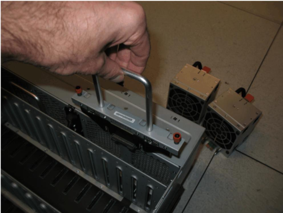
*Figure 176. Remove the FIB from the chassis*
