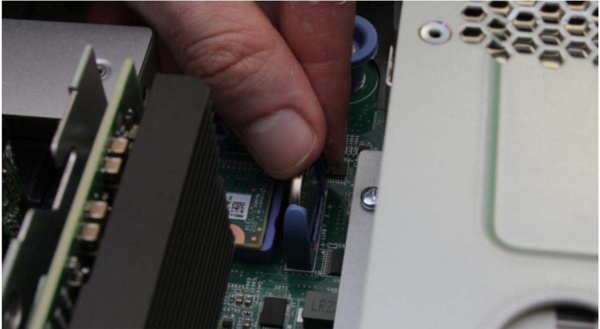
Figure 85. Replacing a CMOS battery
