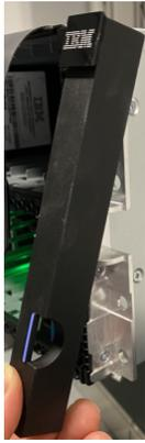
Figure 68. End cap touch point and LED indicators
