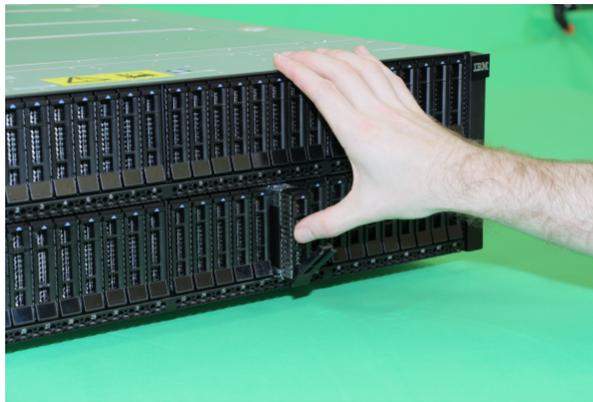
*Figure 73. Inserting the new drive*
