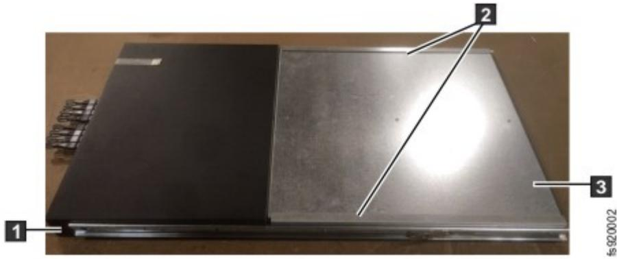
Figure 250. Switch duct rails and ear location
