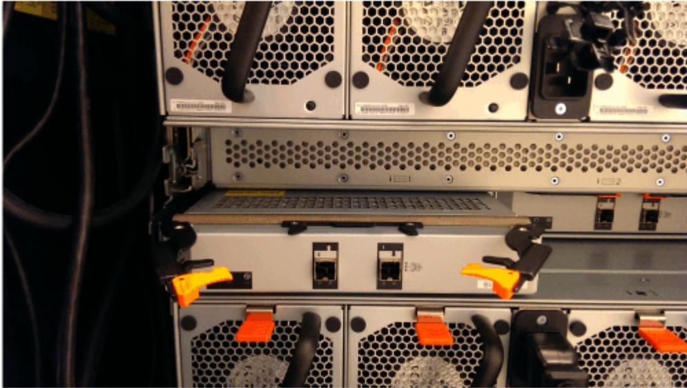
*Figure 165. Removing the expansion canister*
