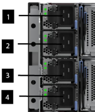
Figure 76. Locate Power Supply Units
