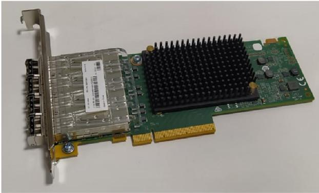
Figure 6. Quad-port 64 Gbps Fibre Channel adapter
