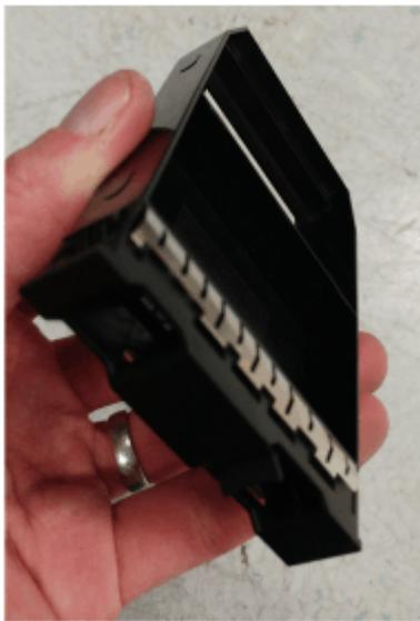
*Figure 75. Correct drive blank orientation*
