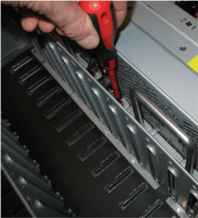
*Figure 175. Loosen the FIB screws*
