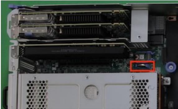
*Figure 84. Locating a CMOS battery*
