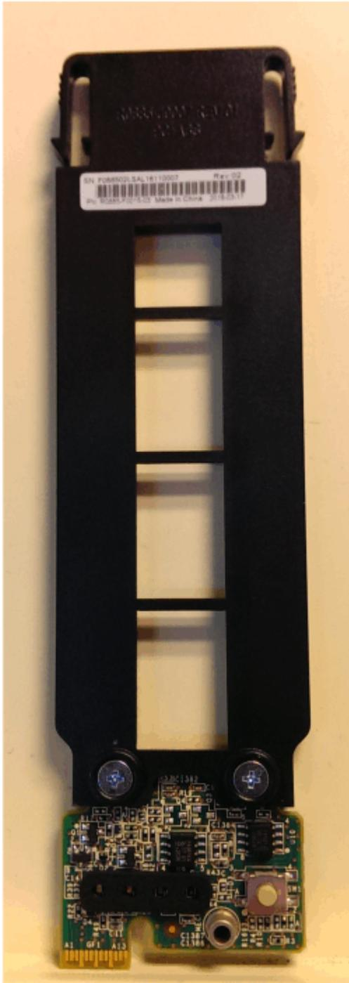
*Figure 162. Display panel assembly*
