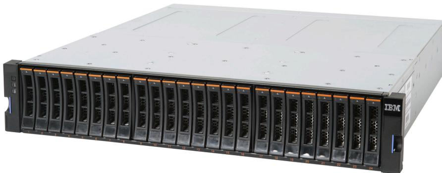
*Figure 19. Front view of an 2U24 expansion enclosure*
