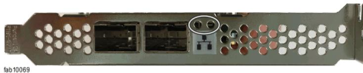
Figure 187. Dual-port 100 Gbps Ethernet adapter host interface adapter ports and LEDs (RoCE)
