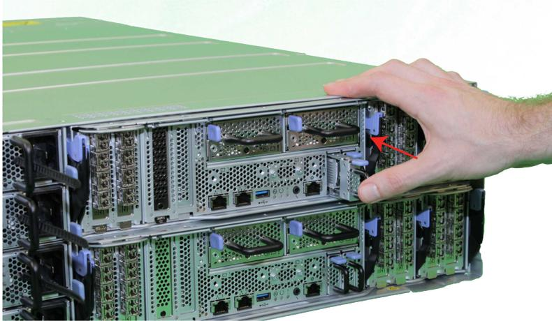
Figure 104. Inserting the boot drive
