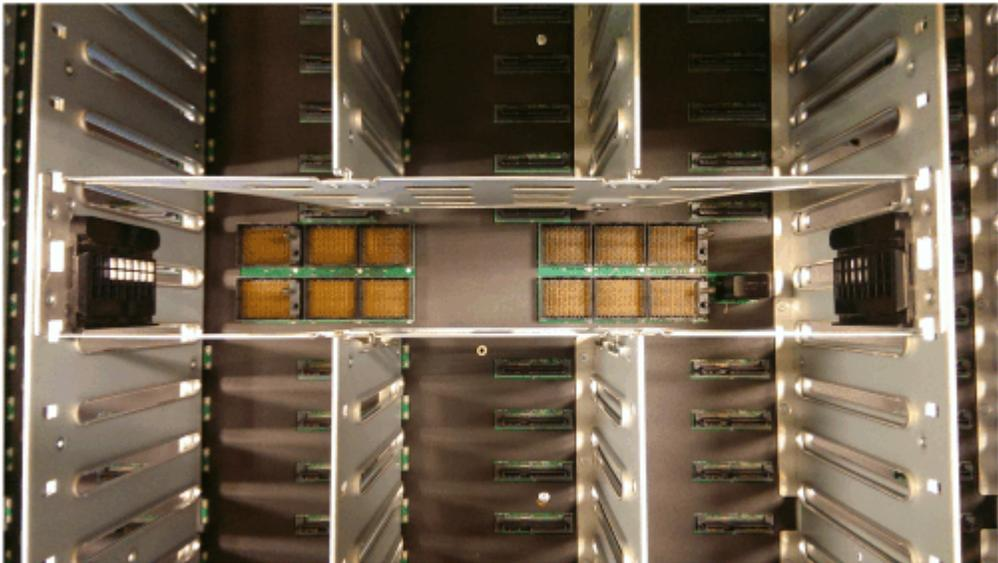
*Figure 147. Secondary expander module connectors*
