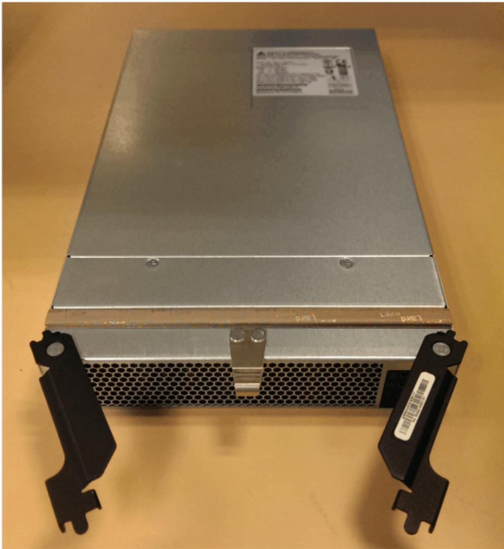
*Figure 158. Preparing to install the power supply*
