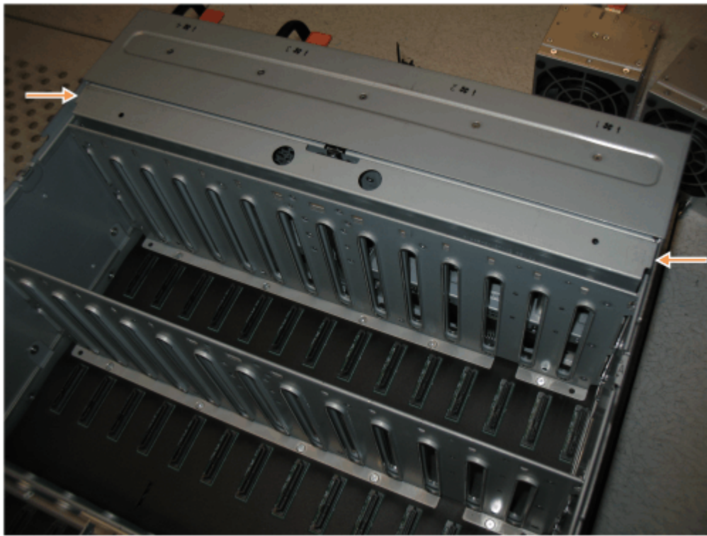
Figure 187. Location of the FIB cover
