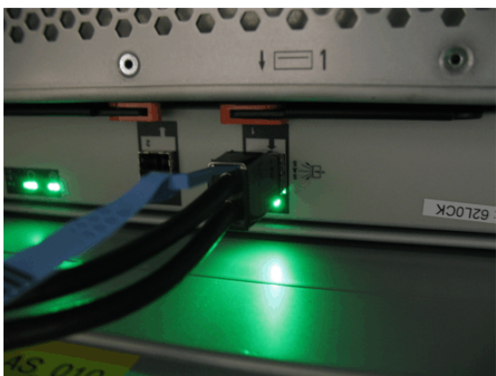
Figure 155. SAS cable correctly inserted into the SAS port
