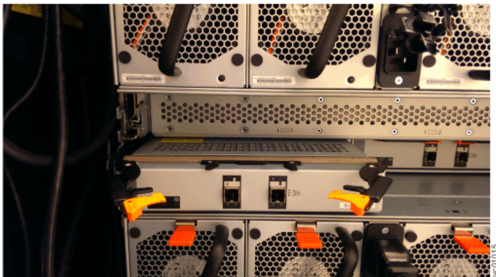
Figure 152. Removing the expansion canister
