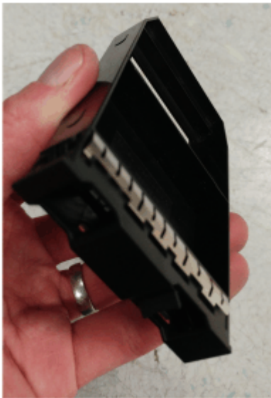
Figure 102. Correct drive blank orientation
