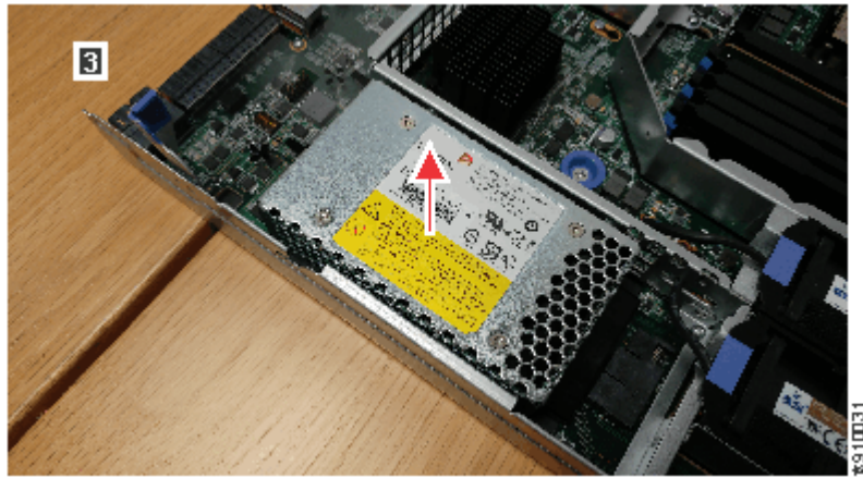
Figure 75. Removing the node battery
