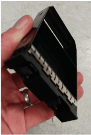
Figure 67. Correct drive blank orientation
