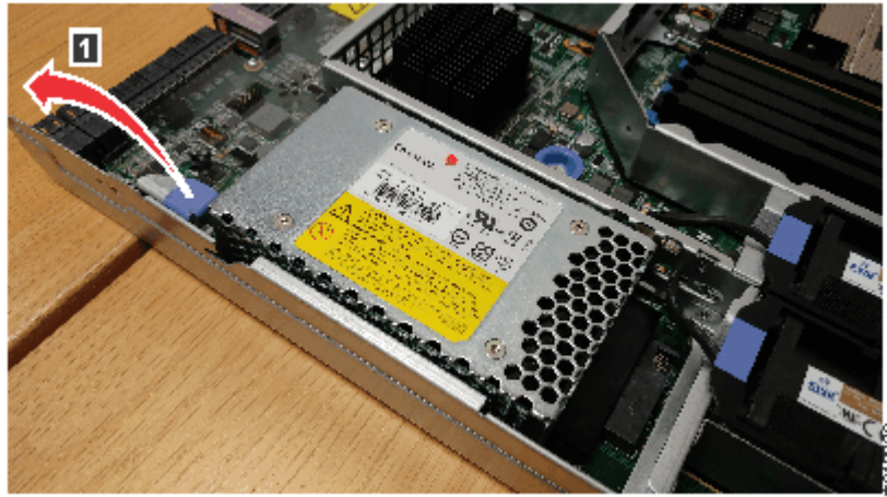
Figure 73. Lifting the latch of the node battery
