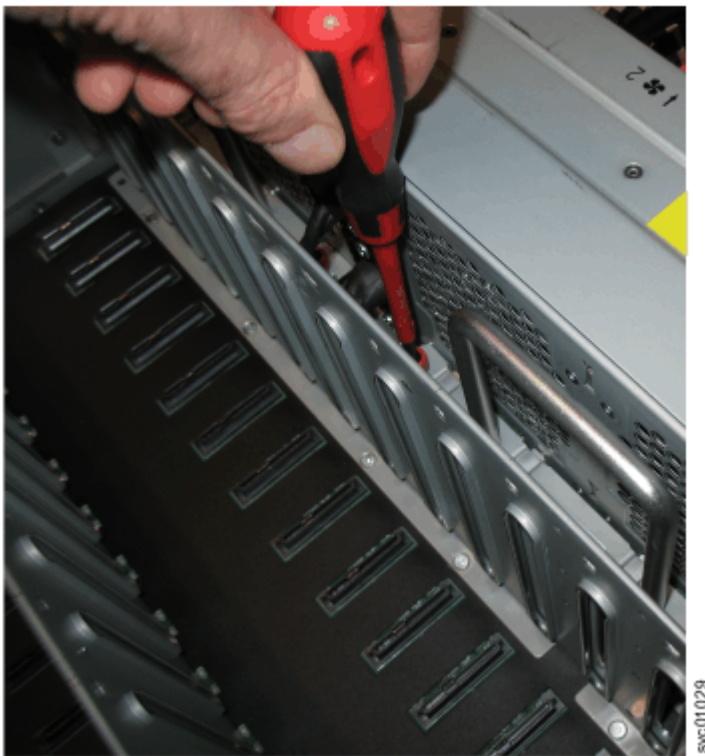
Figure 162. Loosen the FIB screws
