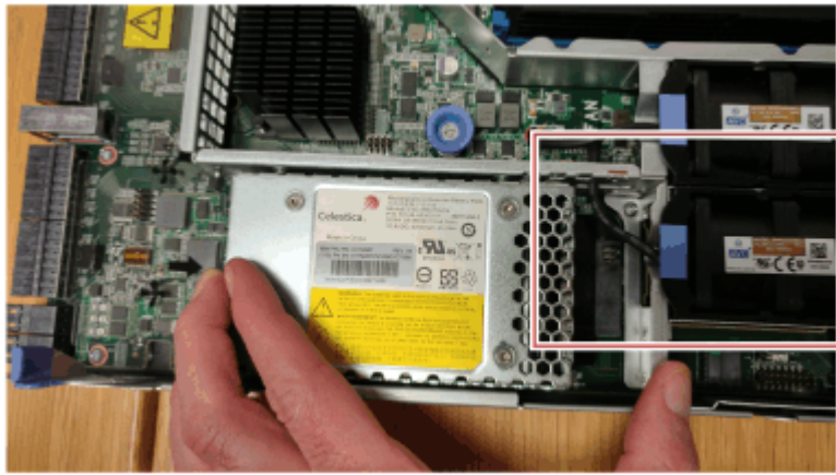
Figure 85. Aligning the cable connector for fan 5
