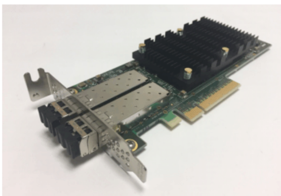
Figure 8. Dual-port 25 Gb Ethernet (iWARP) host interface adapter
