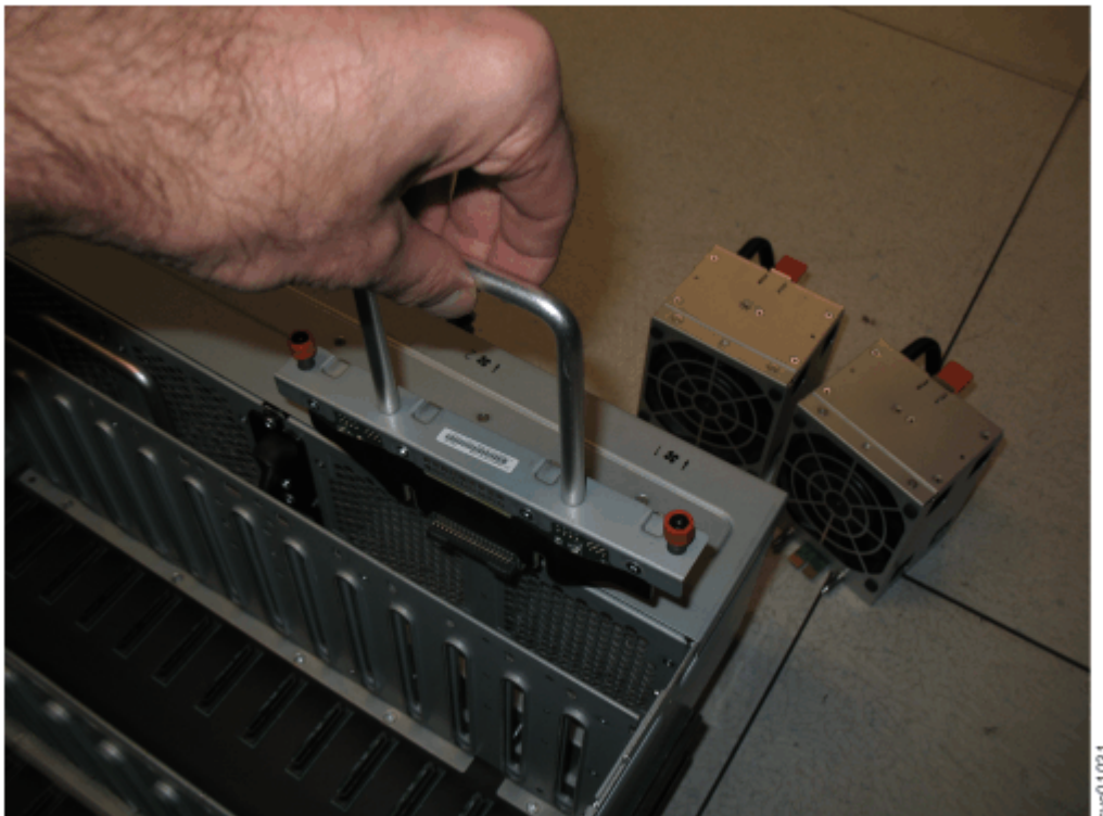
Figure 163. Remove the FIB from the chassis
