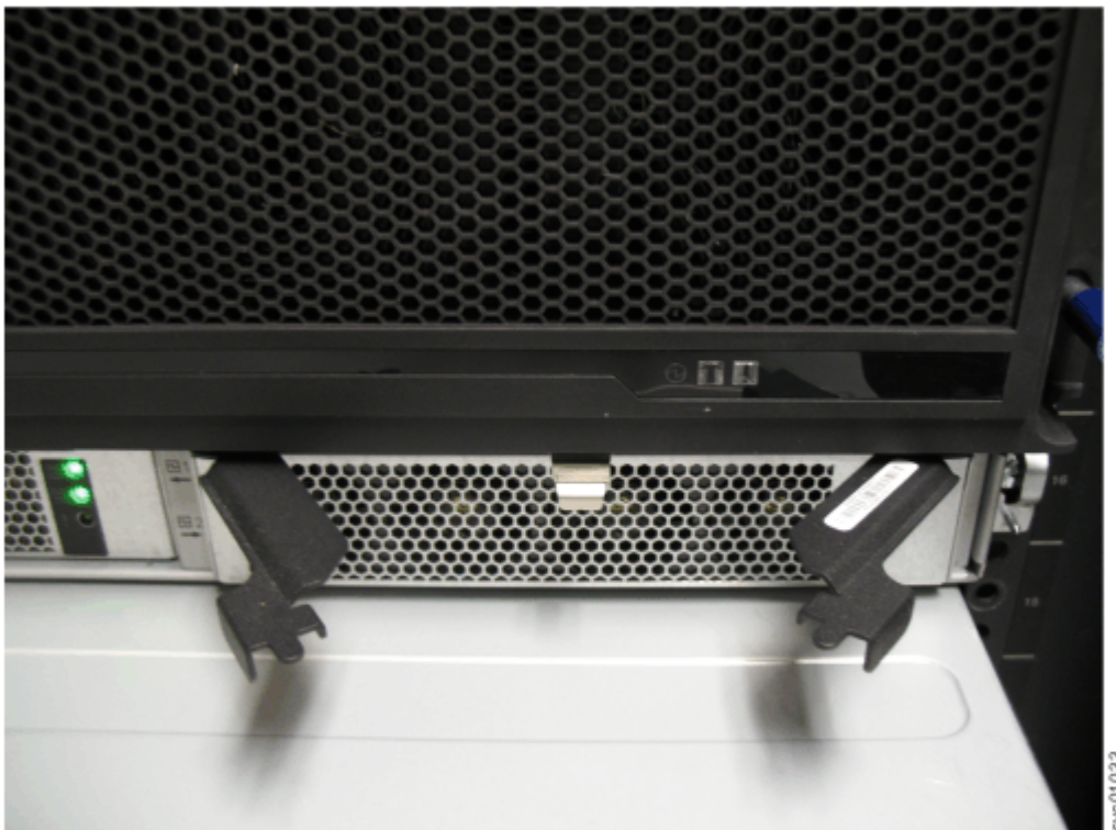
Figure 146. Install the power supply
