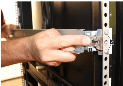
Figure 28. Installing the rear rail bracket
