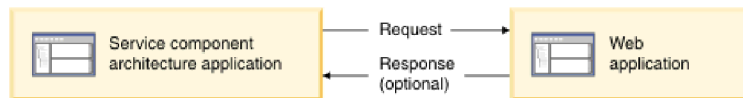
Figure 27. Flow of a request from the SCA application to the Web application
