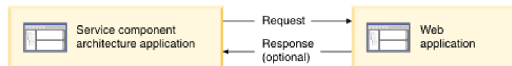
Figure 29. Flow of a request from the SCA application to the Web application
