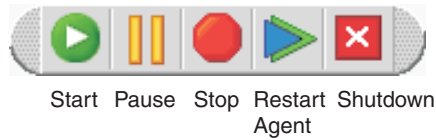
Figure 29. System Monitor, icons for starting, pausing, restarting, or shutting down components
