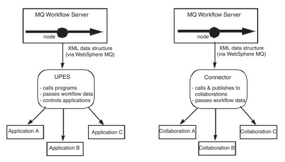
Figure 1. Connector function as an MQ Workflow UPES
