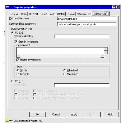
Figure 20. WebSphere MQ Workflow Buildtime: Specifying command-line parameters
