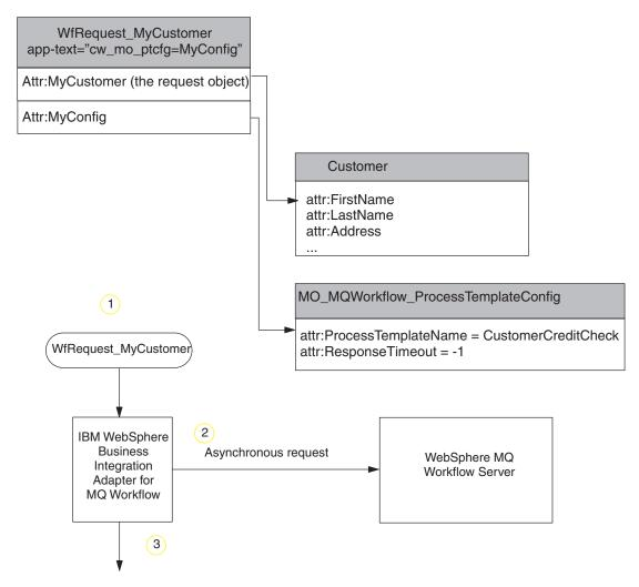
Figure 4. Example asynchronous connector request to MQ Workflow
