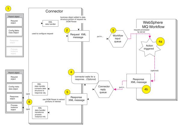
Figure 2. XML API communication mode: Connector-initiated request
