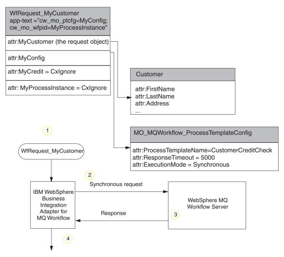
Figure 6. Example synchronous connector request to MQ Workflow
