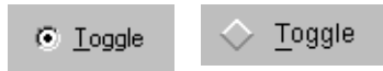
Figure 6.3 A Toggle in Windows95 Look and Feel and a Toggle in Motif Look and Feel
