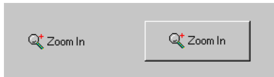
Figure 11.3 Button with Frame Hidden (Left) and with Frame Displayed (Right)
