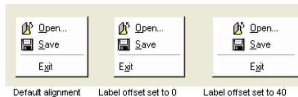
Figure 13.4 Aligning Menu Items Labels
