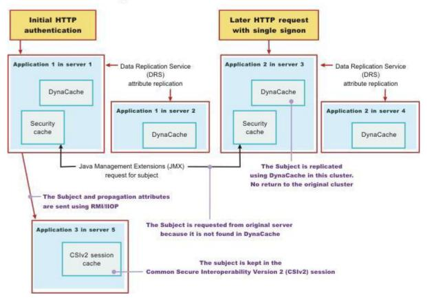
Figure 22. Horizontal propagation
