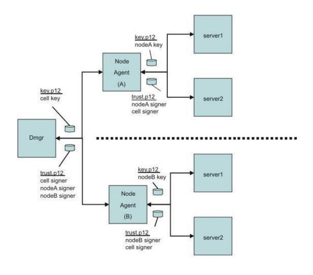
Figure 1: SSL Node Isolation
