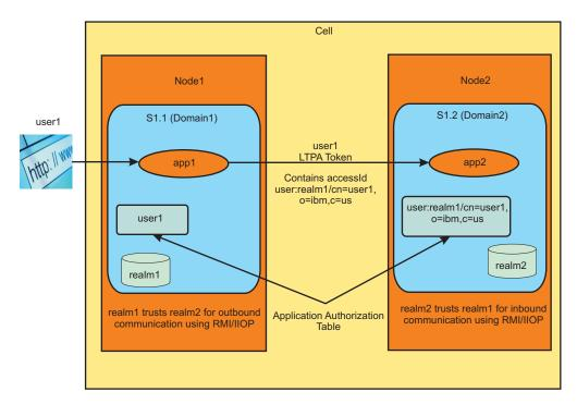
Figure 4. Cross realm communication in a multiple realm environment
