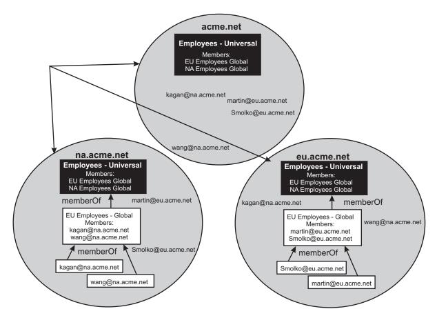
Figure 30. Global catalog (without using referrals). An illustration of a Global Catalog without using referrals
