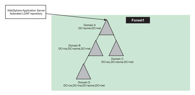
Figure 25. Typical forest configuration. Typical forest configuration.
