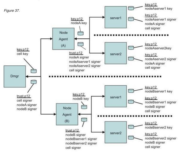
Figure 2: SSL Application Server Isolation
