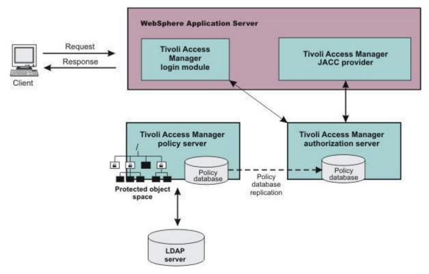
Figure 33. Embedded Tivoli Access Manager client architecture
