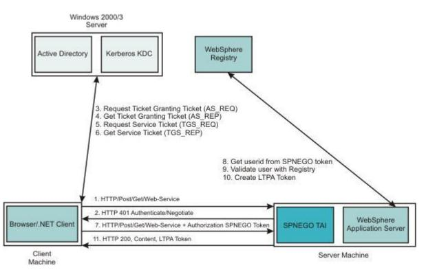
Figure 17. HTTP request processing, WebSphere Application Server - SPNEGO TAI
