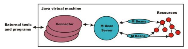
Figure 1. A WebSphere Application Server scripting solution. This figure illustrates the major components involved in a wsadmin scripting solution.
