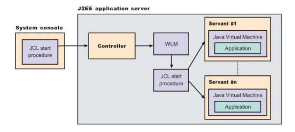
Servers comprise address spaces that run code. A z/OS server has two types of address space: *controllers* and *servants*:
