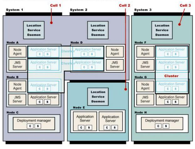
Cells 1 and 3 illustrate Network Deployment configuration cells. Cell 2 is a standalone configuration cell.
