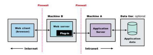
• Scenario 3: Remote Multiple standalone application servers are on one system, and each application server has a dedicated web server on a separate system or logical partition.
