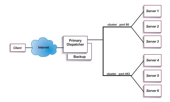
Load Balancer acts as the enterprise's single point-of-presence on the Internet, even if the enterprise uses multiple back-end servers because of high demand or a large amount of content. Availability is achieved through load balancing multiple content hosts and failover support..
