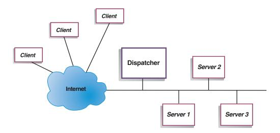
The Dispatcher machine can be installed without making any physical changes to the network. After a client request is directed to the optimal server by the Dispatcher, the response is then sent directly from server to client with no involvement by the Dispatcher.
