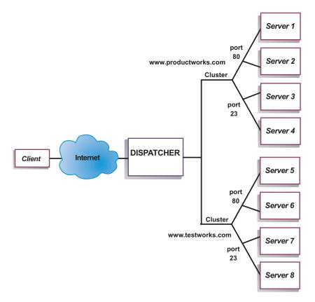
In this example for the Dispatcher component, two clusters are defined with port 80 for HTTP and port 23 for Telnet for each of the sites at www.productworks.com and www.testworks.com.
