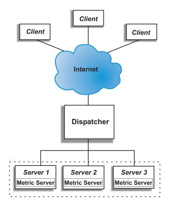
In this example, the Metric Server daemon is installed on each back-end server. You can use Metric Server with the Dispatcher component.
