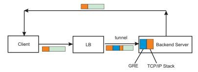
Additionally, this functionality allows you to forward packets to Solaris zones or AIX workload partitions that are on the same host, since Load Balancer can use the existing stack configuration instead of bypassing it entirely.
