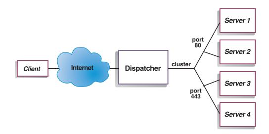
In this example for the Dispatcher component, one cluster is defined at www.productworks.com. This cluster has two ports: port 80 for HTTP and port 443 for SSL. A client making a request to http://www.productworks.com (port 80) goes to a different server than a client requesting https://www.productworks.com (port 443).
