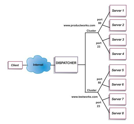
In this example for the Dispatcher component, two clusters are defined with port 80 for HTTP and port 23 for Telnet for each of the sites at www.productworks.com and www.testworks.com.
