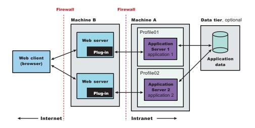
Perform the following procedure to install the plug-ins and configure both Web servers and both application servers.
