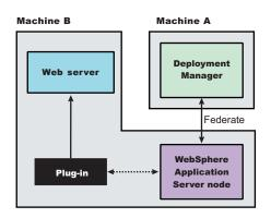
The WebSphere Application Server node on Machine B is the custom node that you create in this procedure. This procedure starts the deployment manager and federates the custom node before installing the Web server plug-ins.
