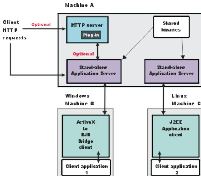
The example shows two types of application clients installed in a topology that uses client applications to access applications and data on Machine A:
