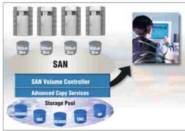
Figure 1. SVC is designed to virtually consolidate capacity from different storage systems, help provide common copy functions and enable data movement without server disruption, while supporting management of diverse storage from a single point.
